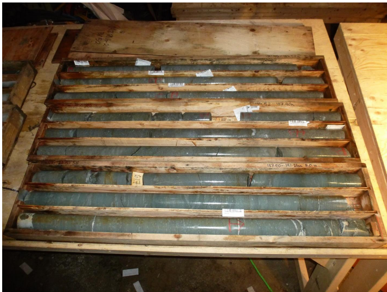
Drill Hole 2016-21: 190.85 - 191.24m (to end of hole): 16 g/t Au and 18.1 g/t Ag
