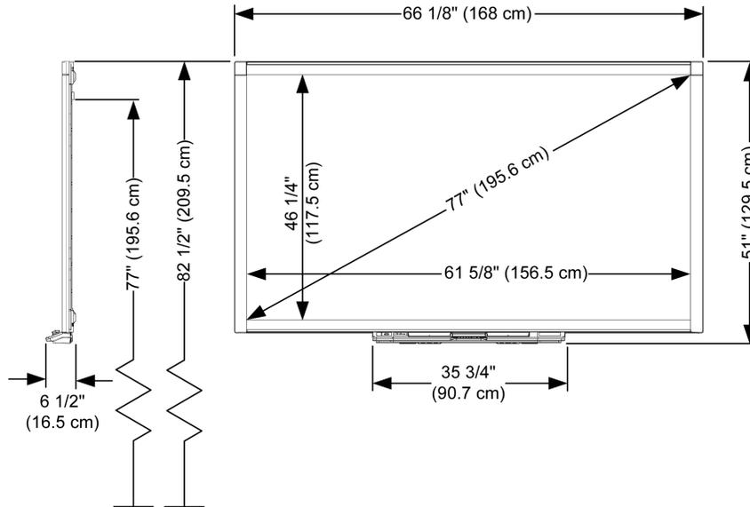
Leave at least 5/8" (1.6 cm) headroom to wall mount the SB880. The distance from the bottom of the wall mount bracket to the top of an installed interactive whiteboard is 6 1/8" (15.6 cm).
