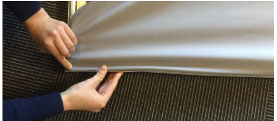
Lay out the fabric skin and start inserting it with its silicone keddar into the rail at the corners of one side. and then at the other corners.
