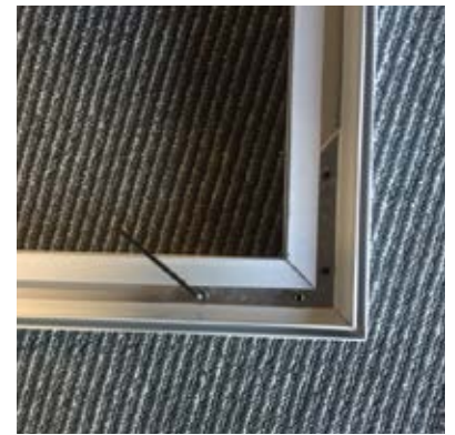
Starting at the top left corner, attach the top and the side profile. Do not tighten the screws until all sides are attached. Ensure all corners are aligned, then tighten all screws using the allen key.
