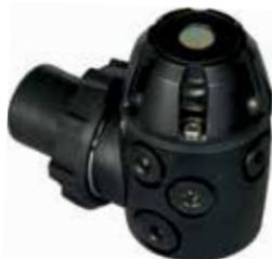
All materials in Xstream Deep are chosen and tested to be optimised for Helium and high flow. This requires special attention to leak tightness, since Helium gas has such a low density. All o-rings are of the highest EPDM quality, and rated for use down to -40°C (-40°F) Deep 1st stage comes in two different versions. One side mounted and one bottom mounted. Both versions are certified to 200m (656 ft) depth, and colour-coded black which in most countries represents a bottom gas mix.
