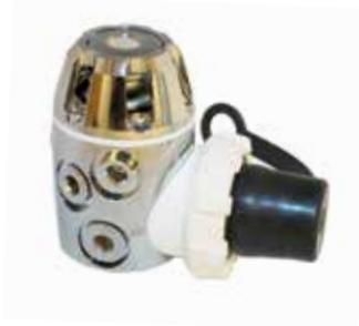
It is identified by the large slots in the cover, allowing the heat energy of the water to reach the spring. The cold from the inside is consequently insulated from the spring, via an insulation barrier and insulating diaphragm. It is constructed without compromise to any detail to prevent cold reaching the sensitive area. Using Poseidon T.D.A, a regulator can free-flow air in fresh water of 0°C (32°F) for at least 10 minutes and afterwards still be completely unaffected.
