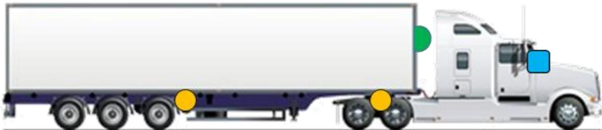
Trailer TPMS 2.0 solutions require some kind of electronic box (●) that identifies them to the tractors they are hooked to so that the trailer tires are monitored by the tractors as well. They also usually have transceivers located near the tires to pick up the TPMS transmissions and forward them to the tractor.
