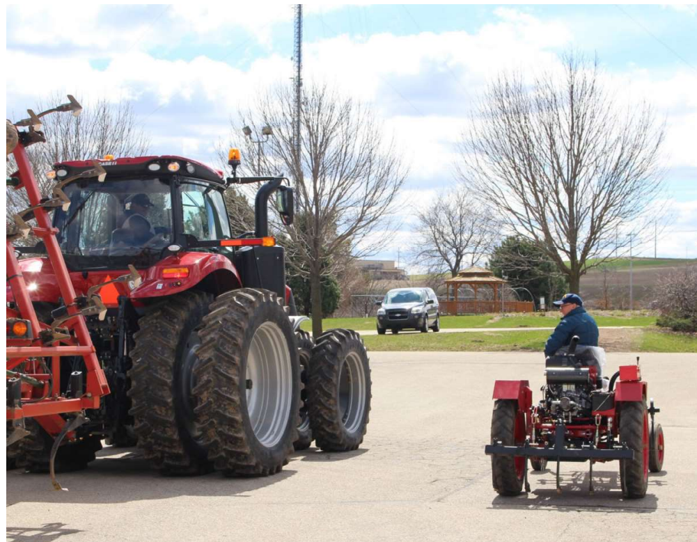
Horace Clemmons compares his Oggún to a typical tractor used in large farming operations. As a single row tractor the Oggún is suited for small farms with 20-60 acres and is designed to be cost effective, simple, rugged and easy to repair.
