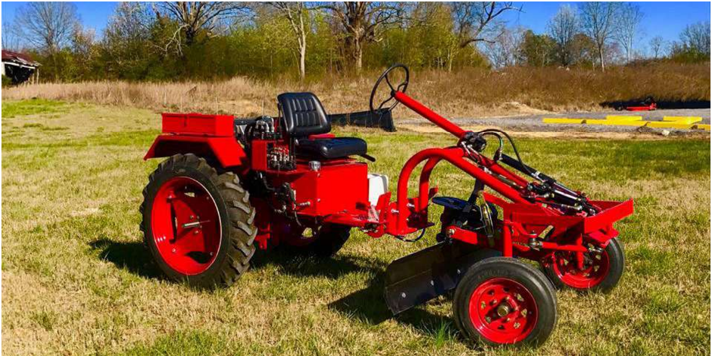
CleBer's Oggún tractor has a simple rear-engine design patterned after the Allis-Chalmers Model G. CleBer's goal is to foster local economic growth in underdeveloped countries by having tractor parts locally sourced.
