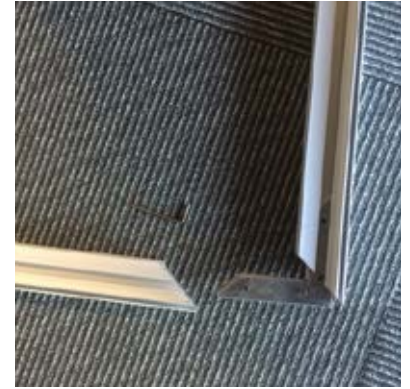
Insert the corner brackets into the tracks of the top and bottom profile of the frame. Screws may need to be loosened to allow brackets to slide into position
