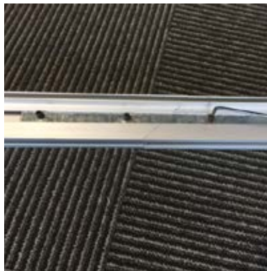
Starting at the top left corner, attach the top and the side profile. Do not tighten the screws until all sides are attached. Ensure all corners are aligned, then tighten all screws using the allen key.
