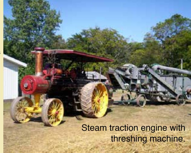
Steam traction engine with threshing machine.
