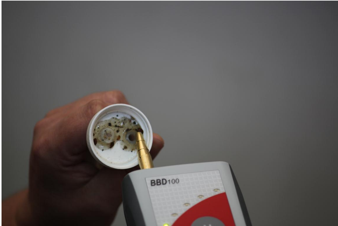
Picture illustrating BBD100 failing to detect 3 bedbugs despite being less than 1 mm away from the live samples
